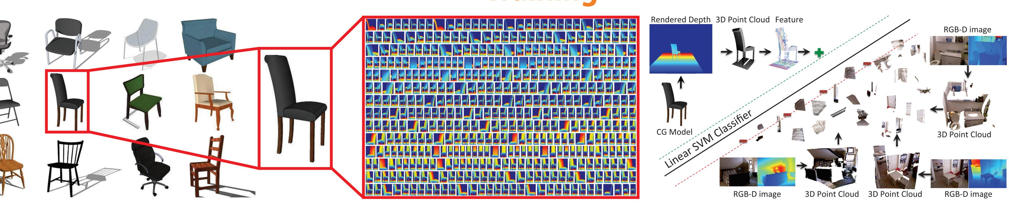
For each object category, we collect the CAD models from the Internet, and for each CAD model, we render depth map from hunderds of viewpoints. For each rendering, a feature vector is extracted from the point cloud and used to train an exemplar SVM using negative data from a RGB-D data set.
