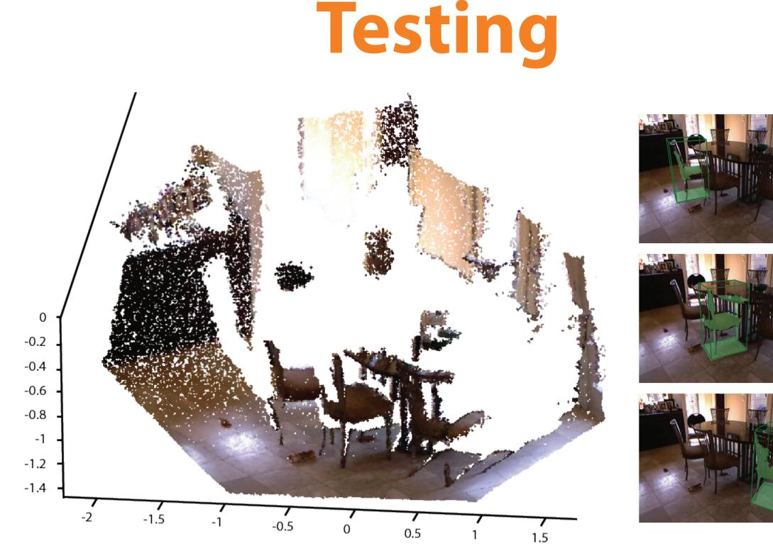
During testing we exhaustively classify each box in the 3D space as chair vs. nonchair, using the Exemplar-SVMs.
